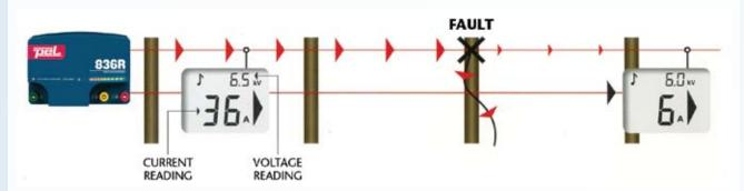
The previous current reading is shown briefly in the top right corner of the screen so that you can compare readings. If the current reading suddenly falls, you have gone past a fault. Retrace your steps to find the fault. Note that after a few seconds the previous current reading will be replaced with the present voltage reading (kV).
